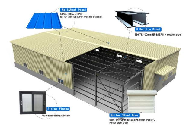
All warehouse complexes and other buildings will be designed using eco-friendly heat & fire-resistant prefabricated material. The rest of the fabrications will use high tensile steel for trusses and beams and aluminum. Floor areas will be coated with anti-slippery coatings and non-reactive floor paint, on self-leveling concrete.
